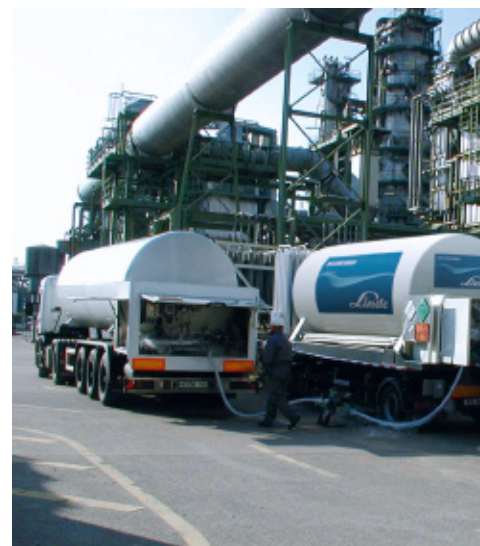
Figure 28: Use of liquid nitrogen to cool down a reactor
