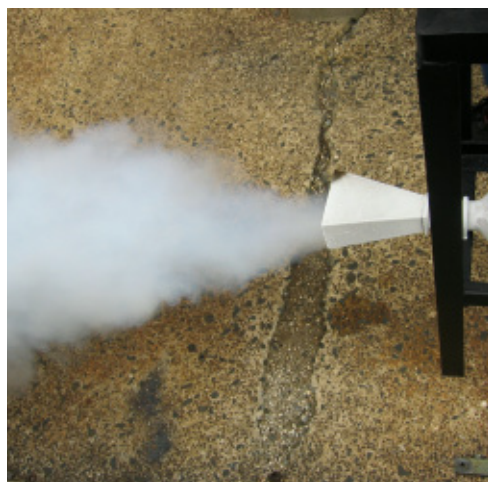
Figure 14: Special nozzle for vaporising carbon dioxide [4]
