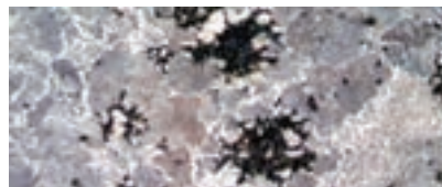
Microstructure of perlitic malleable cast iron (x200)
