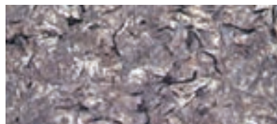
Microstructure of grey cast iron (x200)
