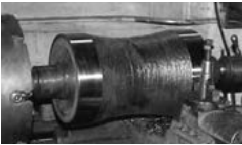
Build-up. Steel mill roll rebuilt to original dimensions - it is being machined prior to service
