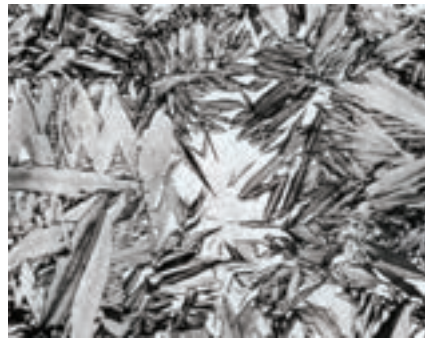
Photomicrograph of martensite
