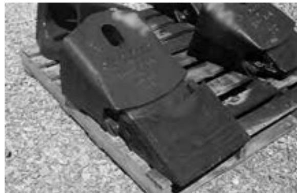
Overlay. Replacement dragline bucket tooth hard surfaced as new equipment
