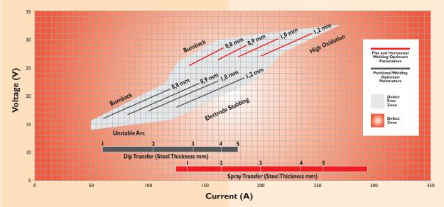
Electrode stick out, contact tip-to-work distance 18 mm for spray, 15 mm for dip, gas flow rate 15 //min Industrial Gases - Shielding Gases
