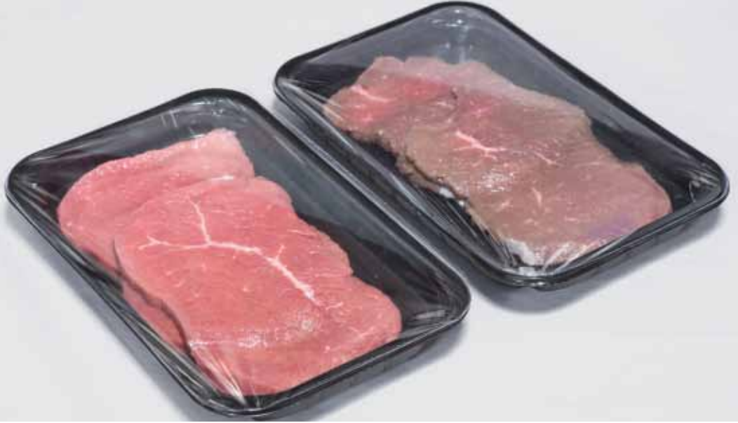
Comparison of two different meat packages – one with modified atmosphere packaging and the other one without
