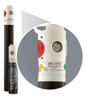
The Afrox Integrated Valve Regulator (IVR) is designed specifically to address the needs of medical practitioners and respiratory therapists for the administration of medical oxygen in portable cylinders. IVR cylinders are ready to use as the valve, regulator, live contents gauge and flow controls are integrated into the cylinder. Therefore no separate regulator is required.
