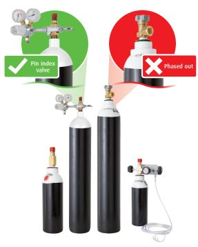
The packaging of medical gases into portable steel and aluminium cylinders is governed by South African National Standard SANS 10019. An amendment to SANS 10019, which was published in 2013, mandates that all medical gas cylinders with a water capacity of 10 litres or less shall be fitted exclusively with a pin index valve.
