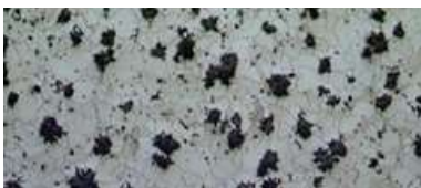
Microstructure of ferritic malleable cast iron (x200)
