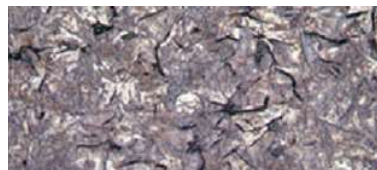
Microstructure of grey cast iron (x200)
