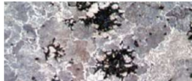
Microstructure of perlitic malleable cast iron (x200)
